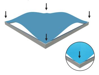
Push the siliconebead into the middle of the run and work your way around the perimeter of the frame until all beading is pushed in properly
